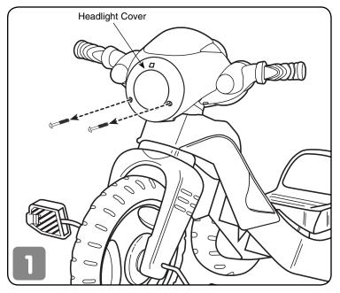
• Loosen and remove the two screws from the headlight cover. Remove the headlight cover.
